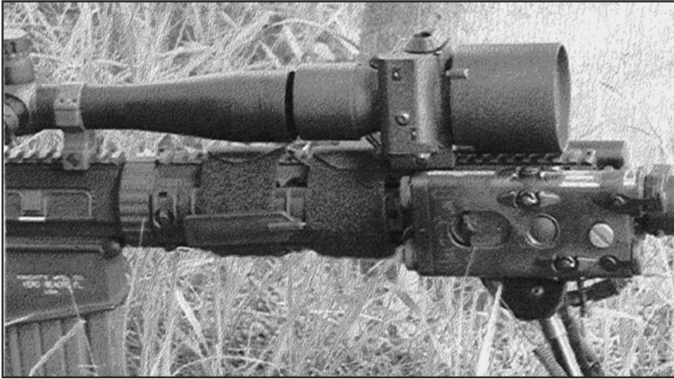
Figure 2-19. Universal Clip-on With AN/PEQ 2
